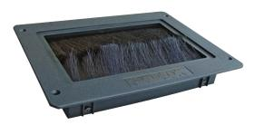
KoldLok seals cable openings in raised floors with an impact-resistant polypropylene grommet insert, which protects cables as they pass through the cut in the raised floor tile, and a double-layer brush closure that seals around cables to prevent cold air from escaping through the hole in the floor.
