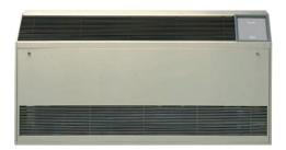
The Liebert DataMate is designed for year-round temperature and humidity control and air filtration in areas where people and electronics must occupy the same space. Its low profile permits floor-mount or wall-mount installation, and requires little or no floor space. The Liebert DataMate provides nominal cooling capacities of 5, 7 or 10.5 kW (1.5, 2 or 3 tons). The system is available in air cooled, water/glycol cooled
